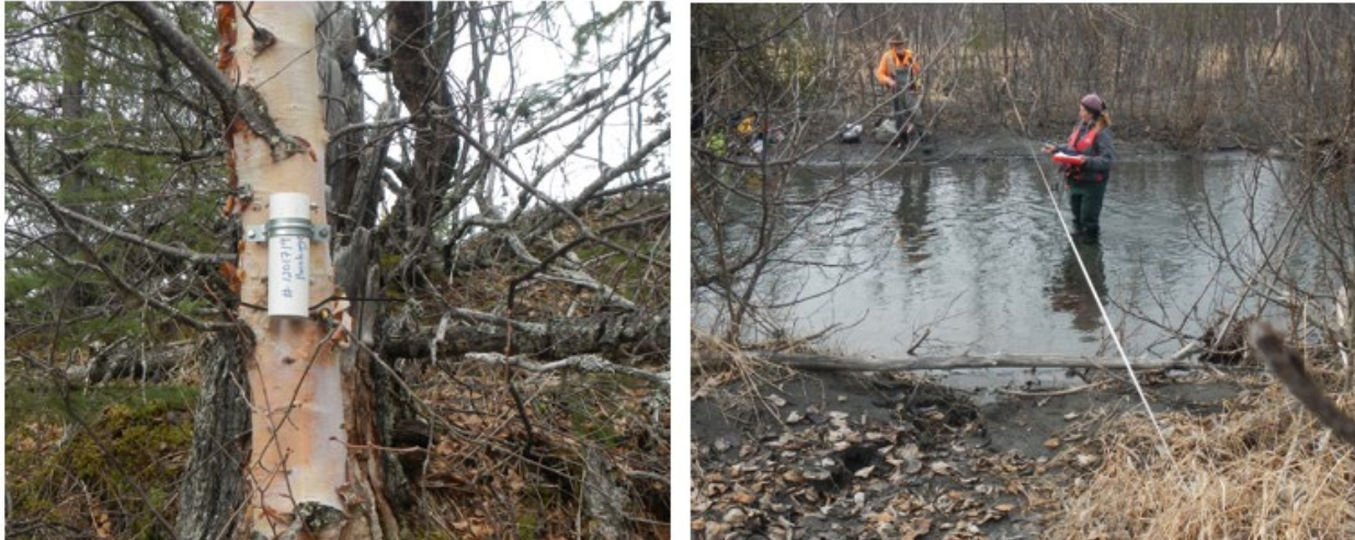
Photo 3-2 Position of barologger installed on a tree, and discharge measurements underway at OCH2.8R-SS-1 in May 2024.
