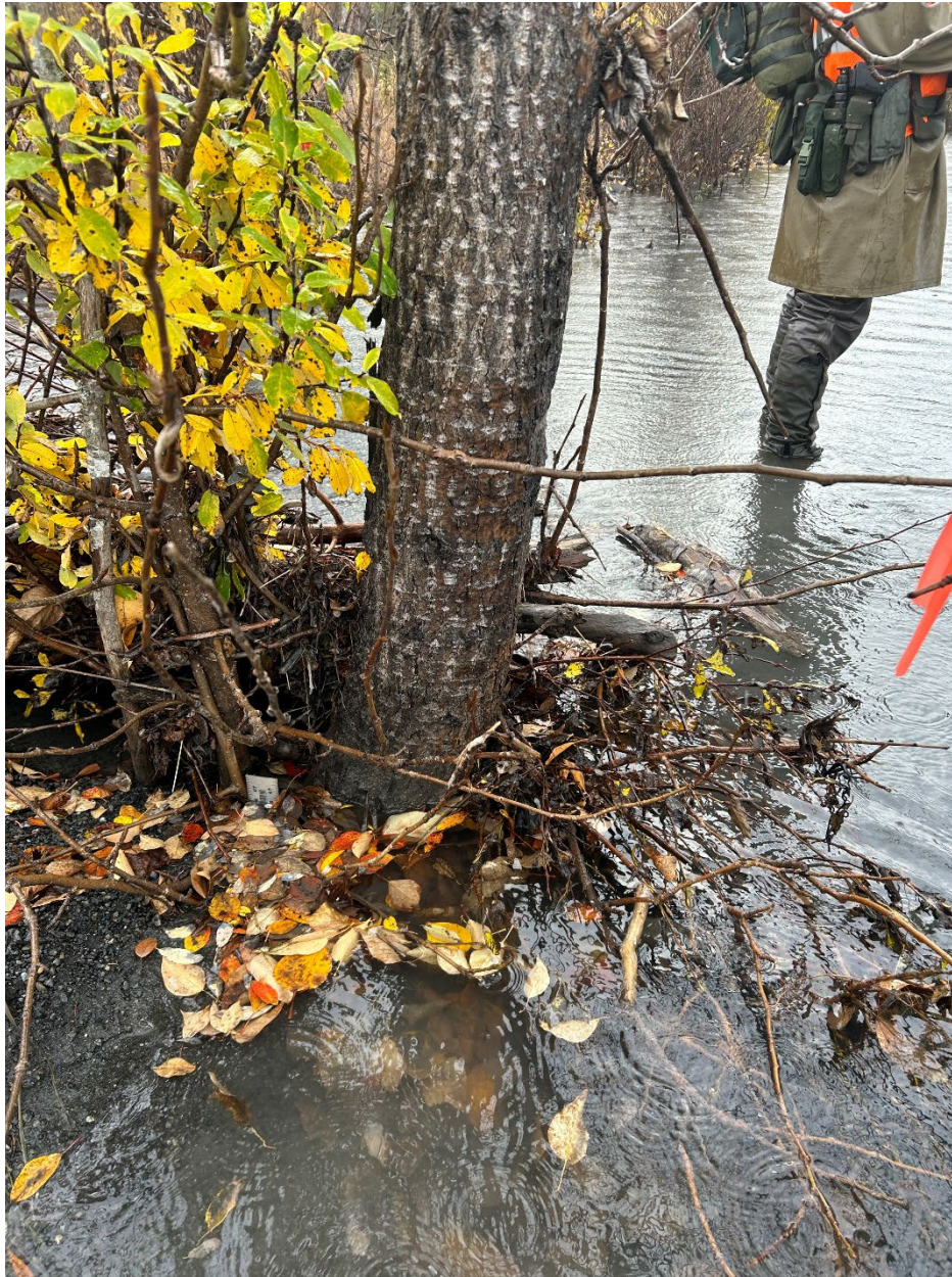
Photo 3-3 Pressure transducer at site OCH2.8R-SS-1 buried after August 7, 2024 flood event. Photo taken September 28, 2024.
